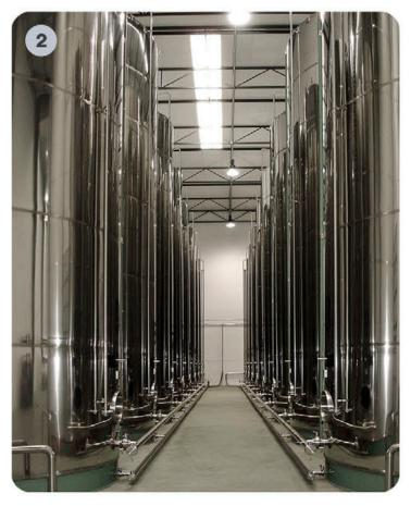
The tanks are completely manufactured in stainless steel and specifically designed for the olive oil industry. The manufacturing process takes place in our factory in Villafranca, where, since 2014, more than 300 tanks have been delivered from to 5 different countries. It was then when the company started new improved systems, leading to an automated and precise assembly process, with high quality welding and a wider range of diameter to cater for our customer's needs.
